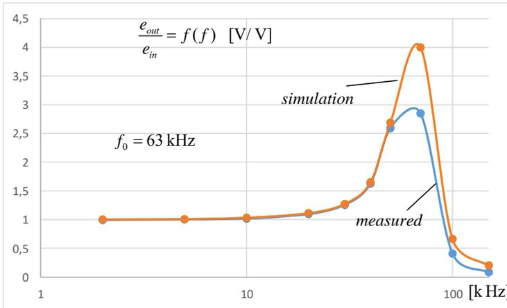
Fig. 6. Amplitude-frequency characteristic of the Rogowski coil (flexible)
