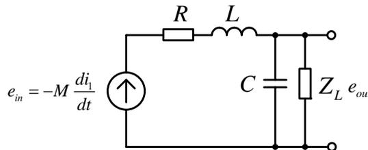
Fig. 2. Substitution scheme of an inductive current transducer
