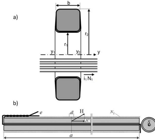
Fig. 1. Inductive transducer with a uniform magnetic circuit
