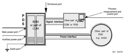
Fig. 1. Internal interfaces of the PDS and examples of ports according to standard [1]
