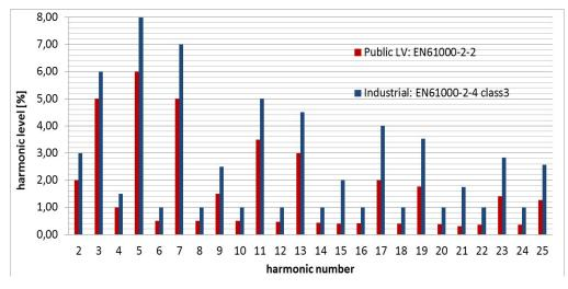
Fig. 2. Minimum requirements for harmonic immunity - compatibility levels
