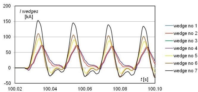
Fig. 9. Current waveforms in the rotor wedges
