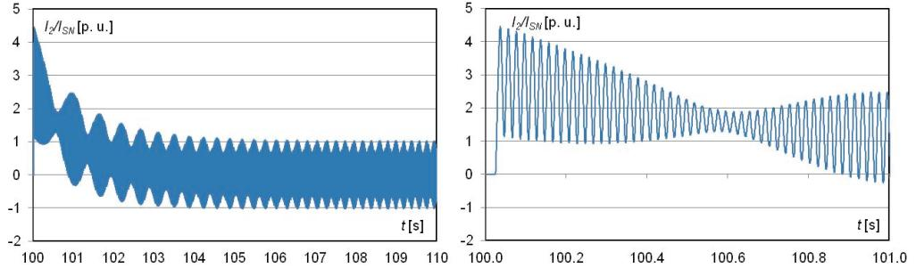
Fig. 6. Negative sequence of stator current
