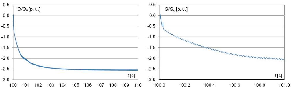
Fig. 11. Reactive power absorbed from the power system
