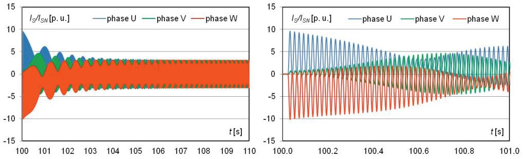
Fig. 5. Stator current waveform in each phase
