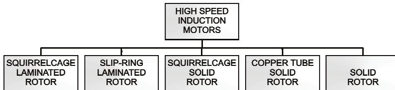
Fig. 2. General classification of high-speed induction motors
