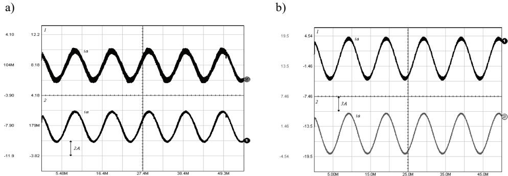
Fig. 9. The current waveform of phase  $A$  for two switching frequencies of voltage generator ( $1 - f_c = 8.33$  kHz;  $2 - f_c = 16.66$  kHz): (a) an economical drive system with half-bridge double voltage rectifier and V-connected inverter supplying 3-phase induction motor; (b) single-phase pulse-controlled rectifier with sinusoidal power line current and three-phase voltage inverter supplying induction motor
