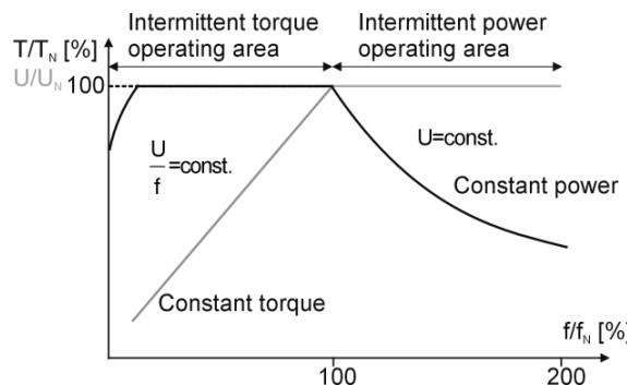
Fig. 1. Allowable change ranges for values of motor torque  $T$  and rms supply voltage  $U$  as a function of inverter output voltage frequency  $f$
