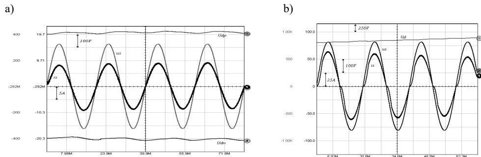
Fig. 10. Voltage waveforms  $u_s$ , a single-phase line current  $i_s$ , DC voltage  $U_d$ : (a) an economical drive system with half-bridge double voltage rectifier and V-connected inverter supplying 3-phase induction motor; (b) single-phase pulse-controlled rectifier with sinusoidal power line current and three-phase voltage inverter supplying 3-phase induction motor
