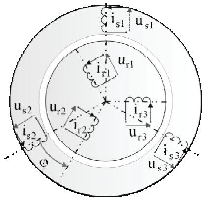
Fig. 3. Model of a three-phase induction machine
