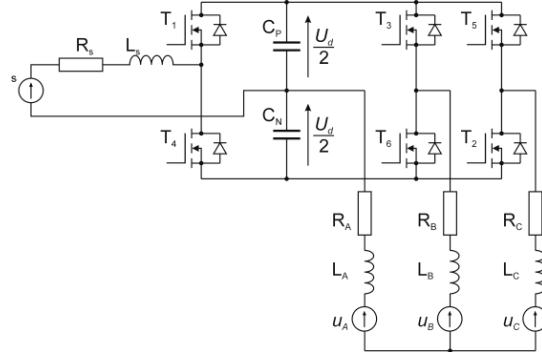
Fig. 6. An economical drive system with half-bridge voltage multiplying rectifier and V-connected inverter supplying an induction motor
