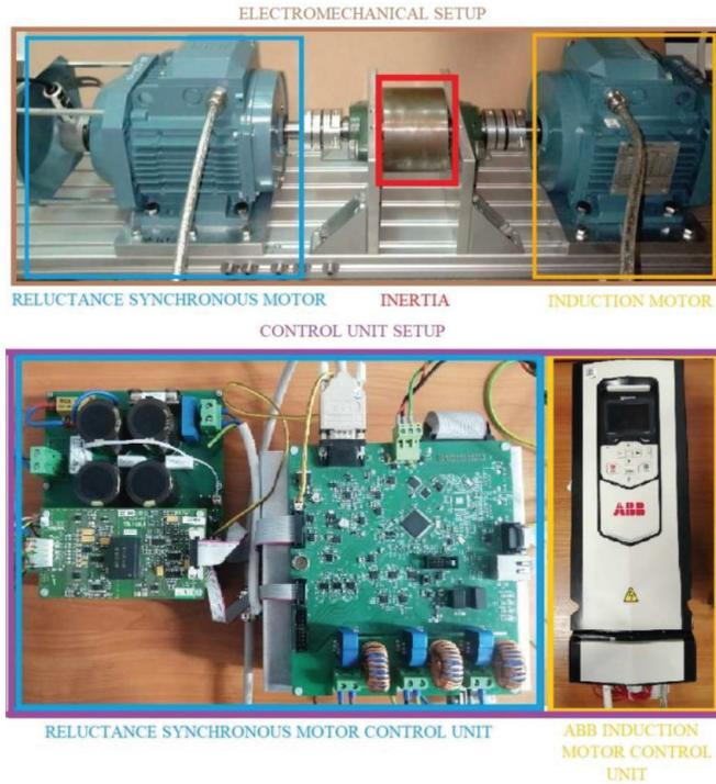
Fig. 4. The experimental setup with RSM drive and IM load drive.
