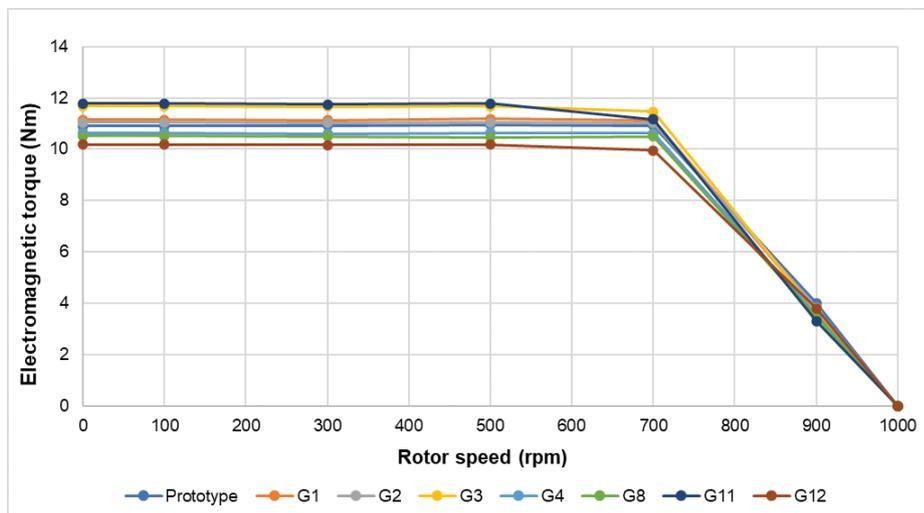
Fig. 6. Electromagnetic torque vs speed characteristics for all analysed motor models.
