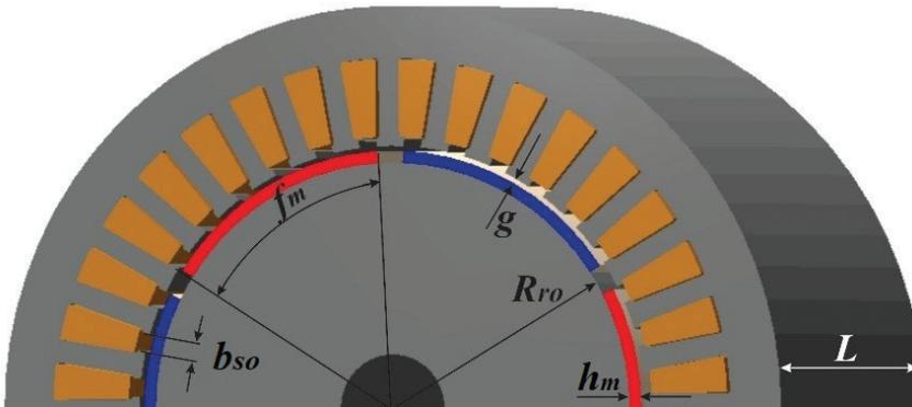
Fig. 1. PMSM cross-section and optimisation parameters presentation. PMSM, permanent magnet synchronous motor.
