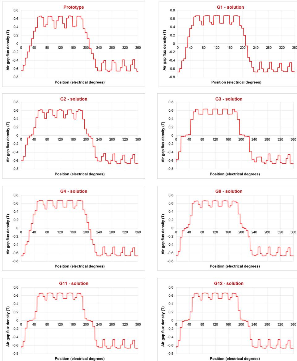
Fig. 4. Air gap flux density distribution for all analysed motor models.
