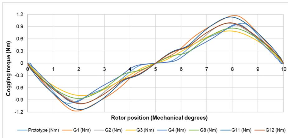
Fig. 5. Cogging torque distribution for all analysed motor models.
