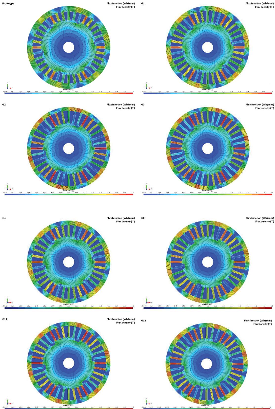
**Fig. 3.** Magnetic field distribution for all analysed motor models.
