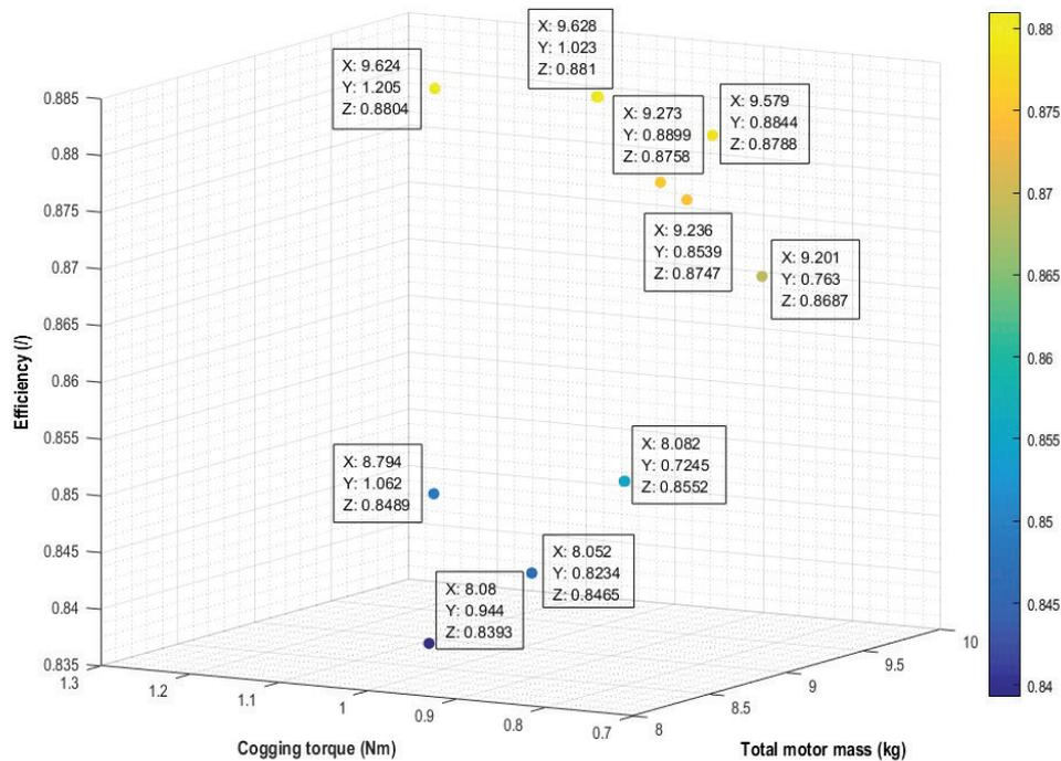
**Fig. 2.** Comparative presentation of the optimisation solutions (X axes is total motor mass, Y axes is cogging torque, and Z axes is efficiency).
