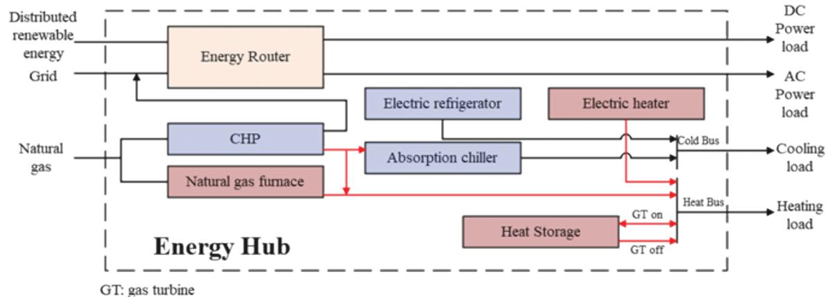
Fig. 17. The topology of an energy router Li et al. (2020).
