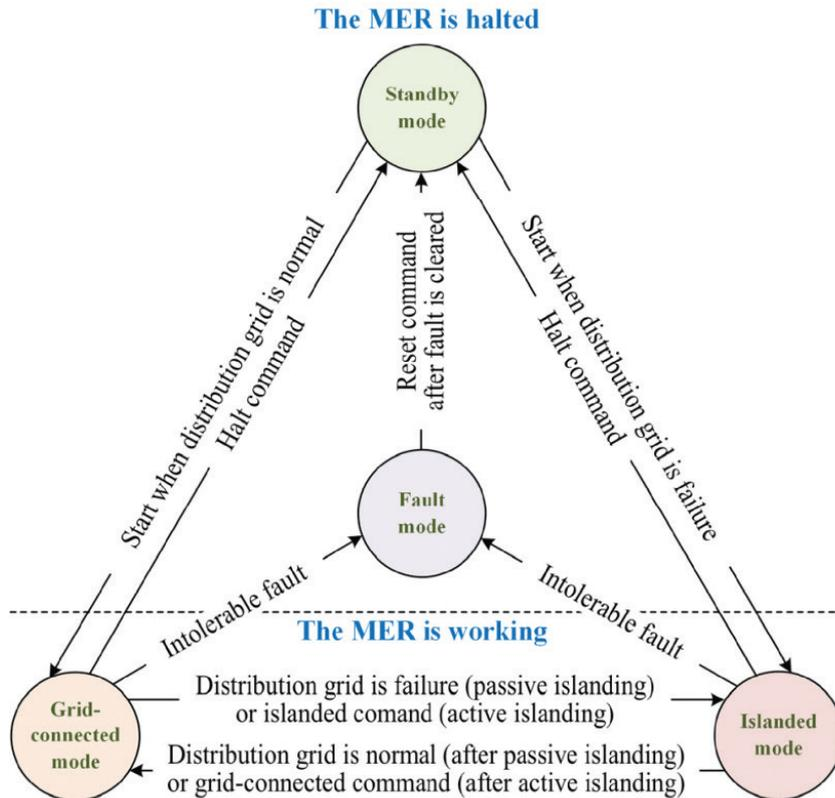
**Fig. 6.** Operation mode transition of MER Liu et al. (2019). MER, multi-port energy router.
