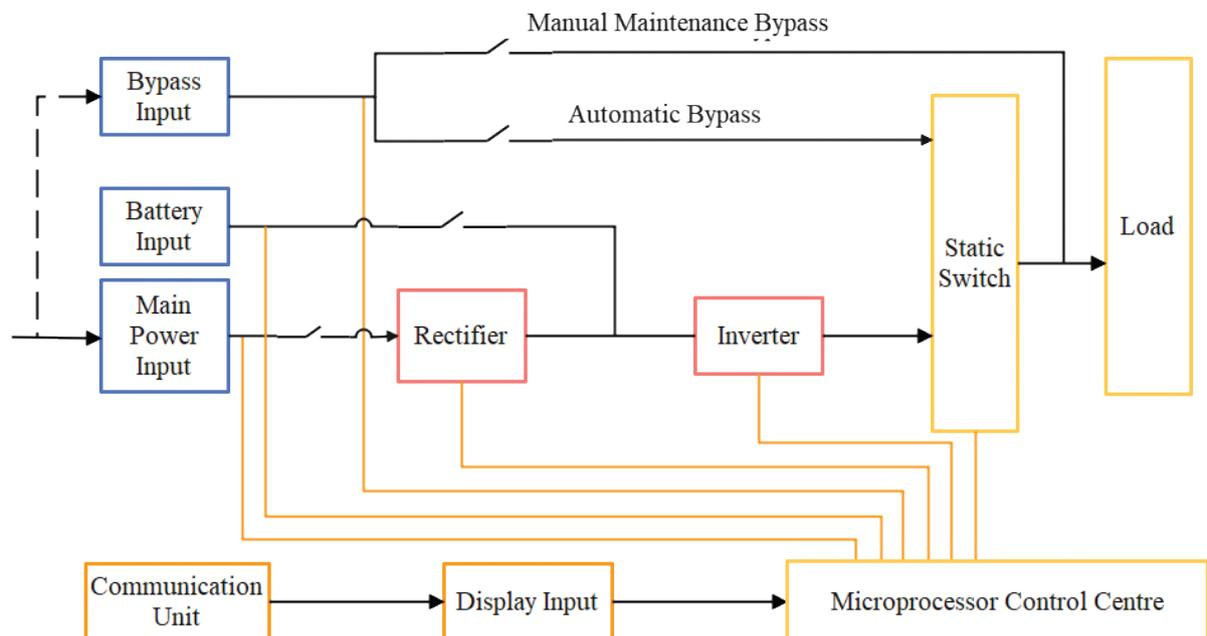
Fig. 3. The whole function diagram of EPS. EPS, emergency power supply.
