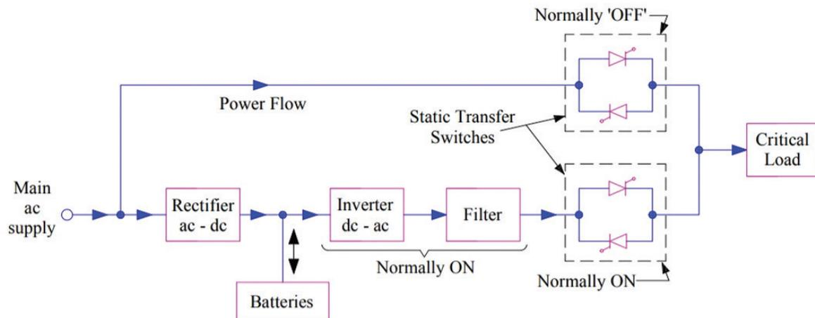
Fig. 2. Working principles of UPS (Electrical Concepts, 2022). UPS, uninterrupt power supply.
