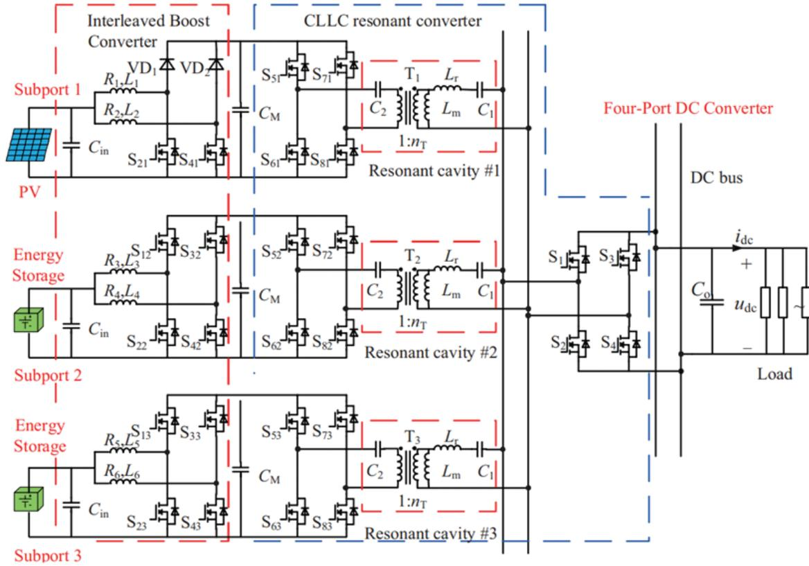
**Fig. 15.** DC micro-grid structure diagram of photovoltaic energy storage with FPIC (Liang et al., 2020). FPIC, Four-port isolated DC/DC converter.
