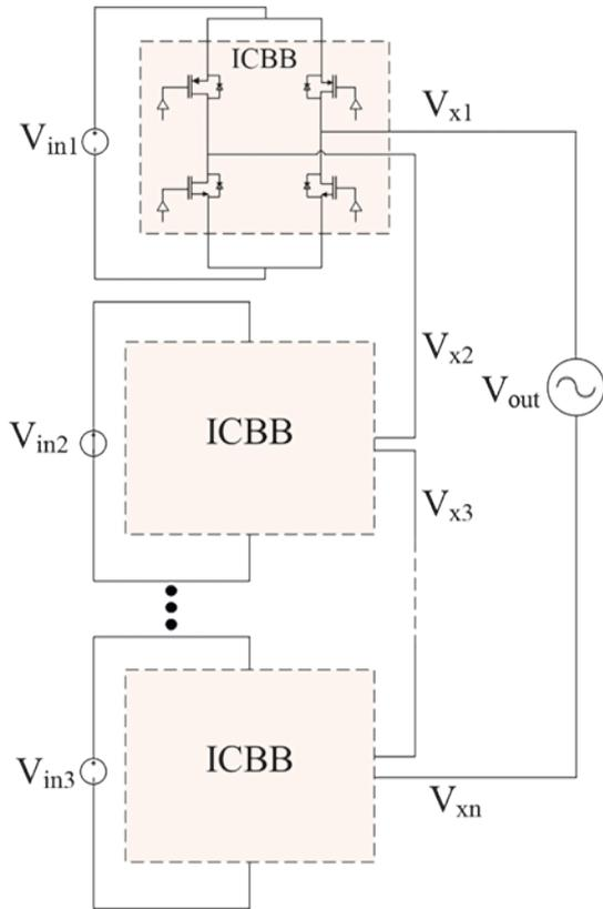
Fig. 10. Multilevel inverter implementation utilising ICBB modules Ahsanuzzaman et al. (2017). ICBB, integrated circuit building block.
