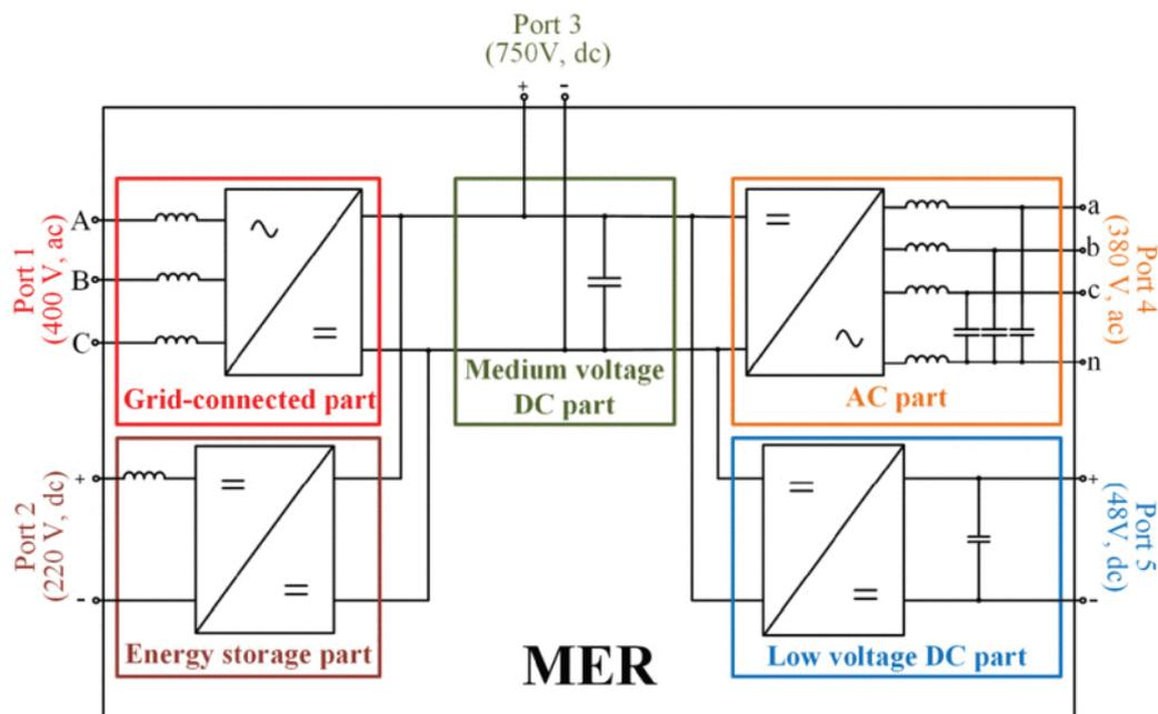
Fig. 5. Structure of MER Liu et al. (2019). MER, multi-port energy router.
