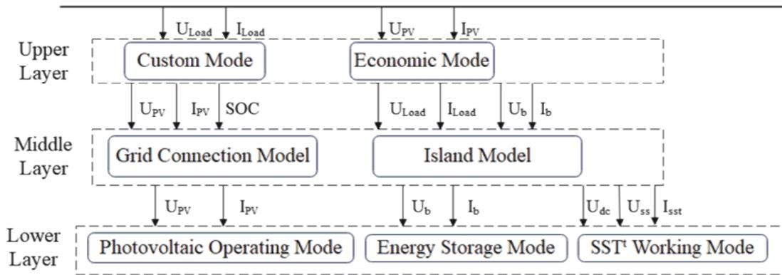
Fig. 8. Hierarchical control system. SST, solid state transformer.
