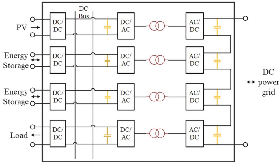
Fig. 7. Topology of energy router based on power electronic transformer.
