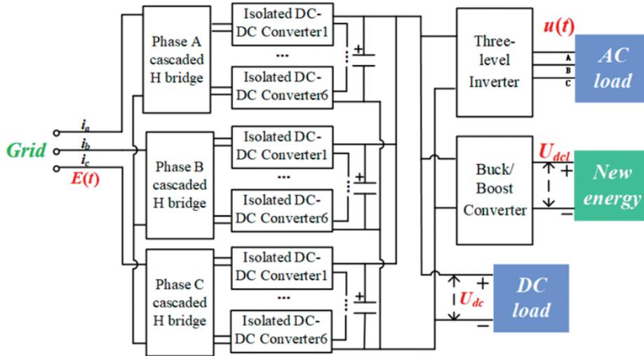
Fig. 11. A topology of MER Chi et al. (2021). MER, multi-port energy router.
