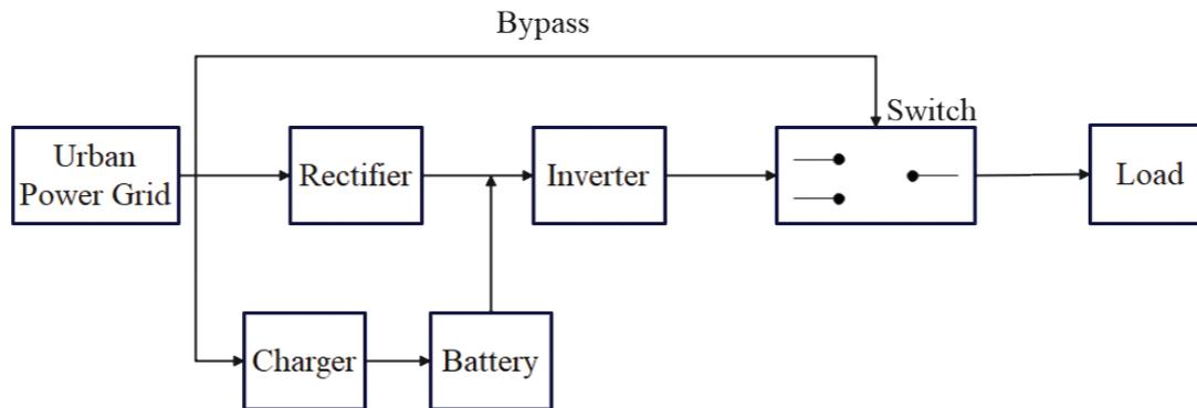
Fig. 4. Function diagram of distributed power.
