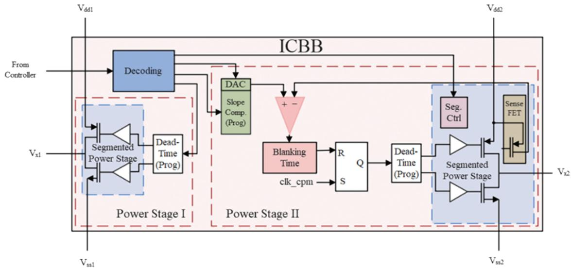
**Fig. 9.** Block diagram of low-power ICBB Ahsanuzzaman et al. (2017). ICBB, integrated circuit building block.
