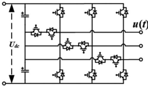
Fig. 14. Topology of DC/AC converter Chi et al. (2021).
