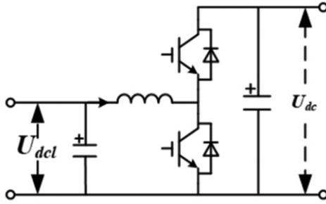
Fig. 13. Topology of DC/DC converter Chi et al. (2021).
