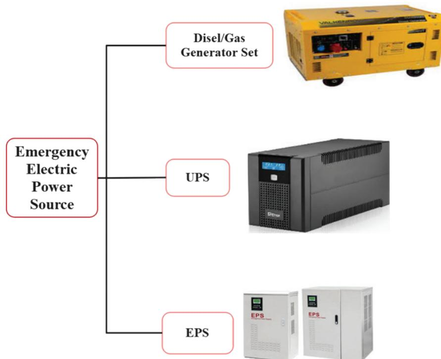
**Fig. 1.** Different kinds of emergency electric power sources. EPS, emergency power supply; UPS, uninterruptible power supply.
