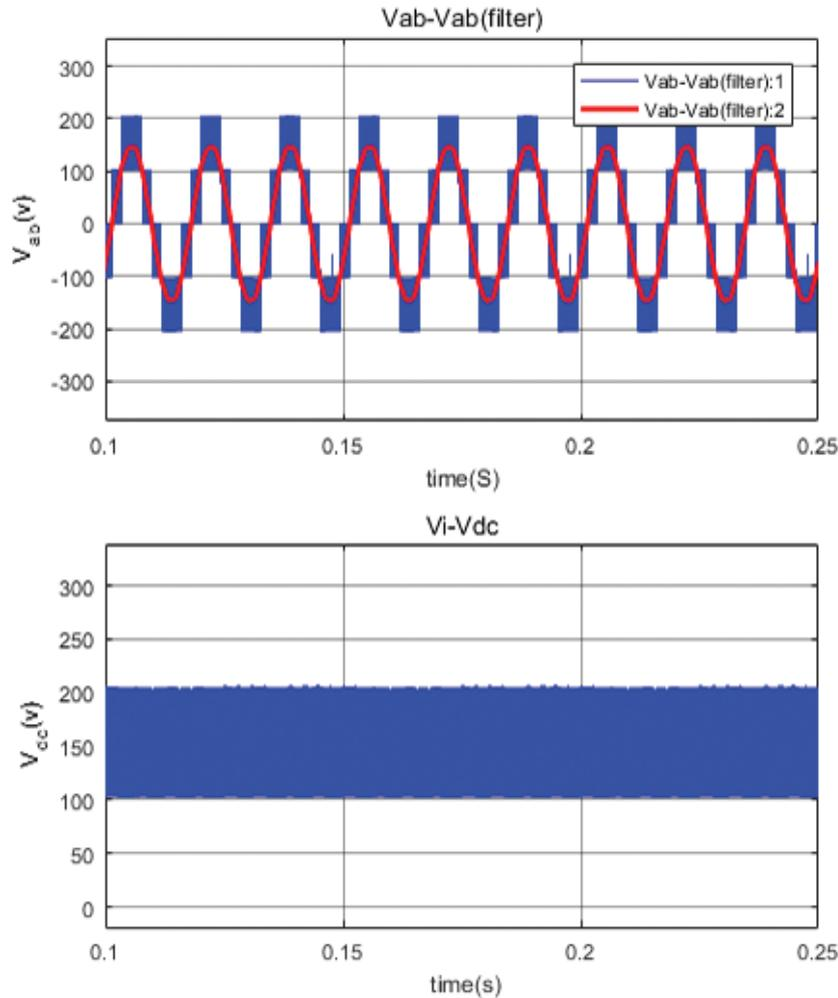
**Fig. 8.** Output voltage waveform and DC link voltage at  $M = 0.8$ .
