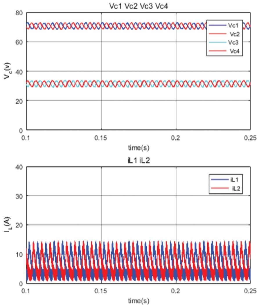
**Fig. 9.** Voltage waveform of capacitors and inductors at  $M = 0.8$ .
