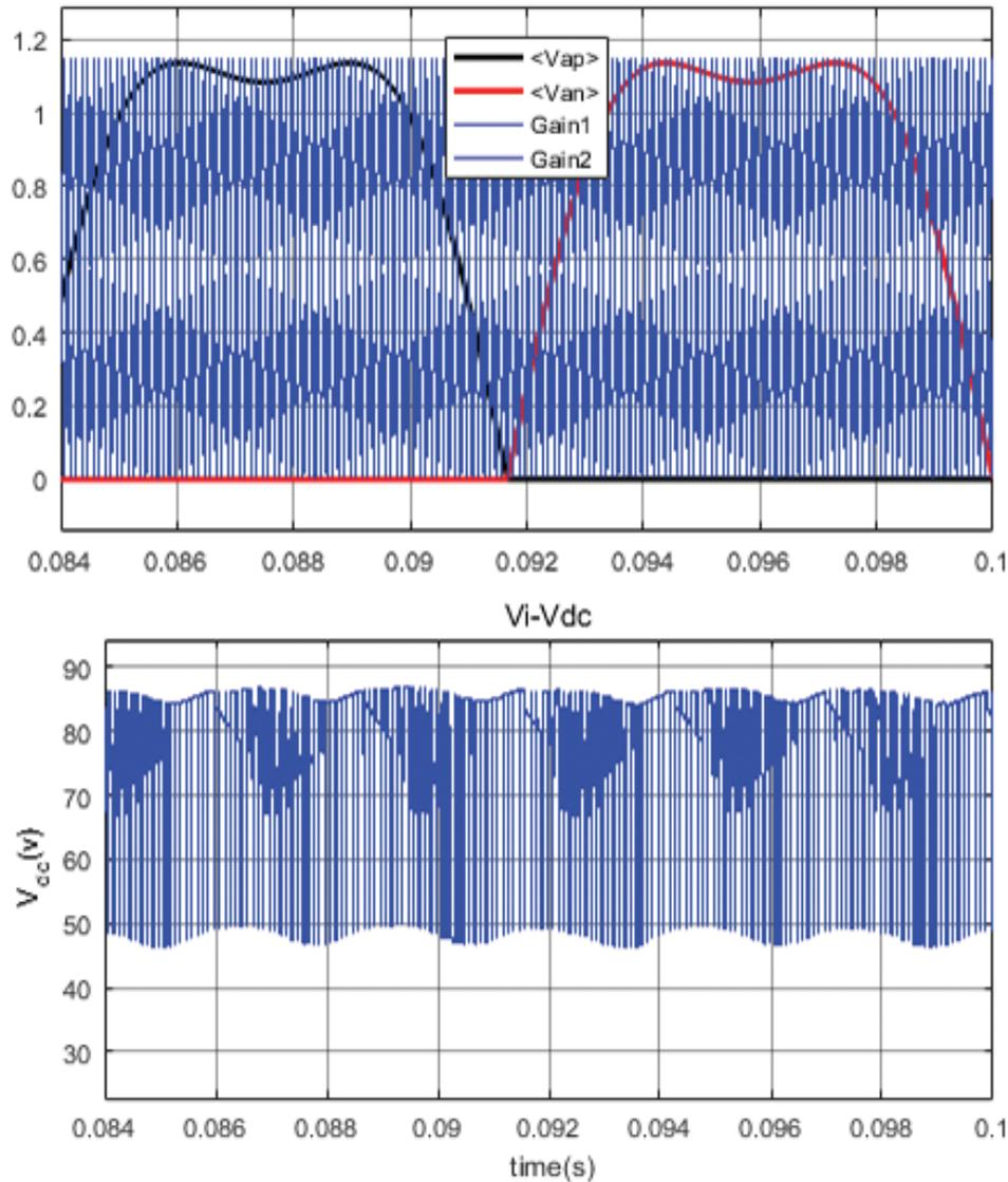
**Fig. 13.** a-phase modulation signal waveform and DC link voltage at  $M = 1.15$ .
