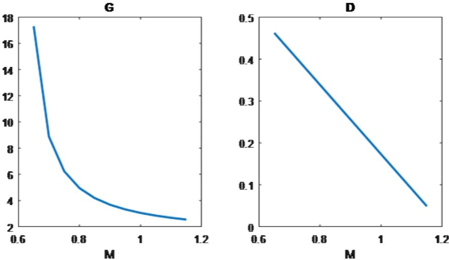
Fig. 6. Shoot-through state waveforms in terms of diode cycle and voltage gain with M changes.
