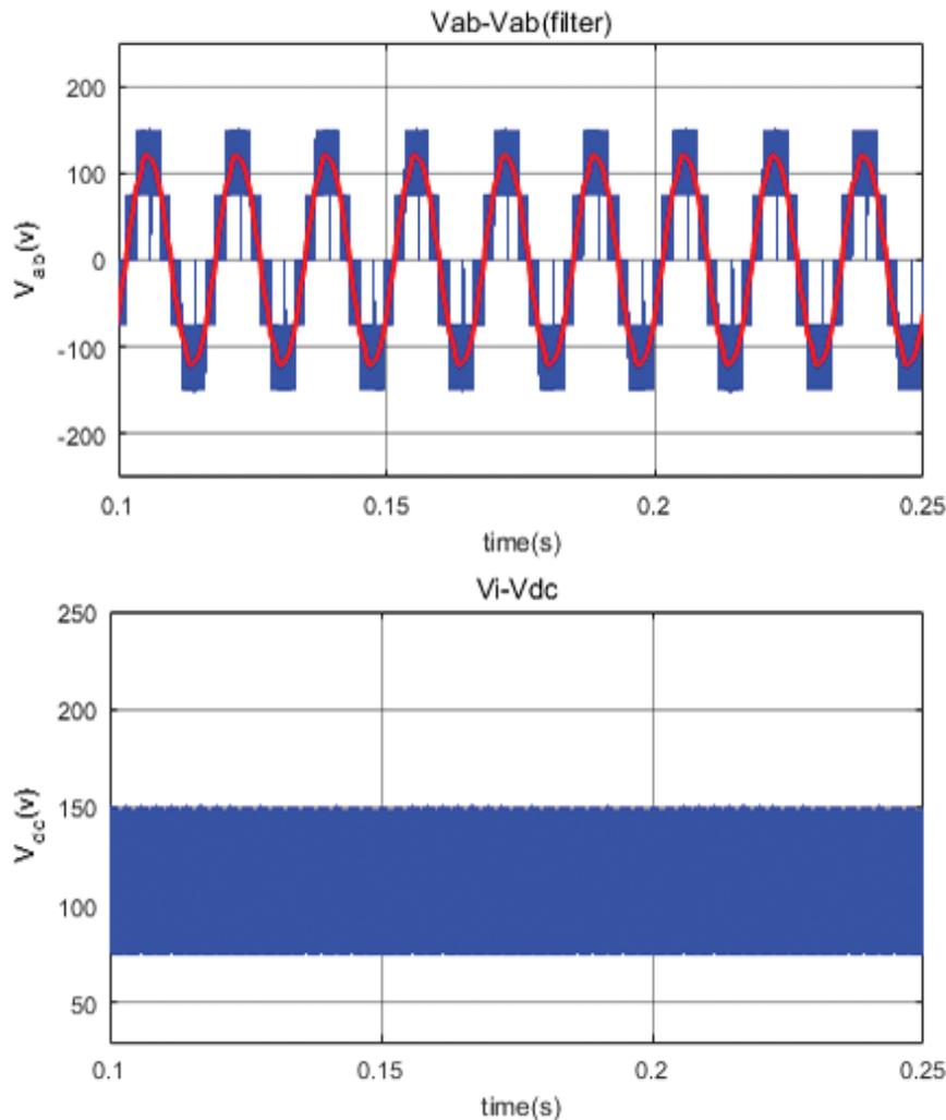
**Fig. 11.** Output voltage waveform, DC link voltage at  $M = 0.9$ .
