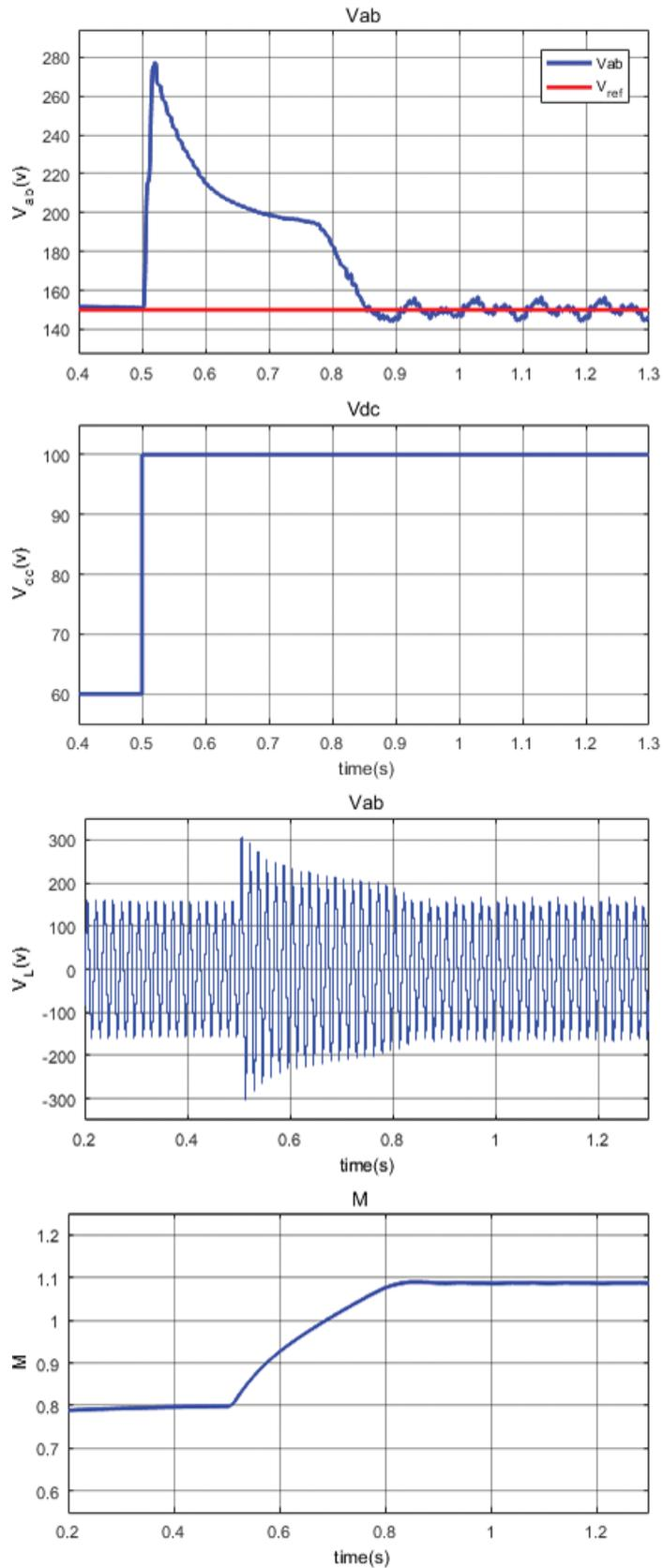
**Fig. 14.** Load voltage amplitude waveform, input voltage, load voltage and amplitude modulation for load voltage change when DC link voltage in islanding mode increases from 60 to 100.
