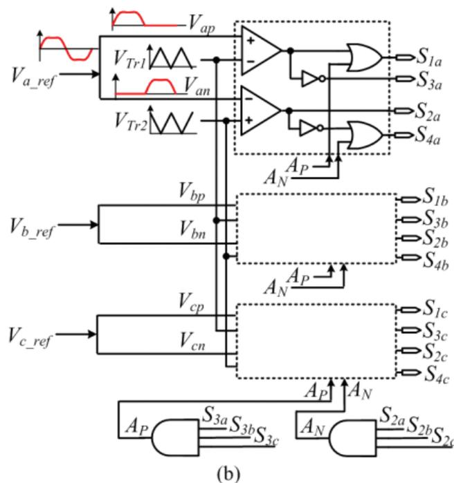
**Fig. 4.** Modified modulation strategy logic circuit for three-level MZS-NPC inverter (Strzelecki, 2006). MZS-NPC, modified Z-source neutral-point clamped.
