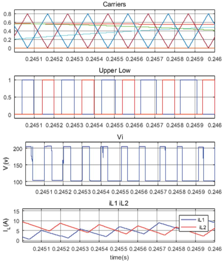
**Fig. 10.** Three-phase modulation signal, upper and lower shoot-through state signal, DC link voltage and inductor current at  $M = 0.8$ .
