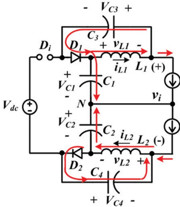
Fig. 3. Converter equivalent circuit in the non-shoot through state.
