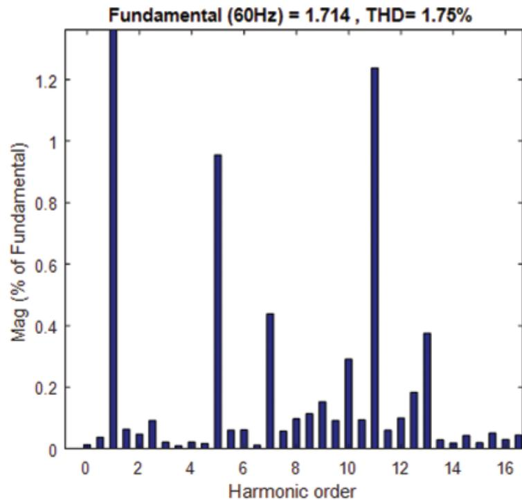
Fig. 15. Frequency spectrum of a-phase current. THD, total harmonic distortion.
