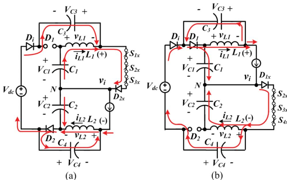
Fig. 2. Converter equivalent circuit in (a) upper shoot-through state and (b) lower shoot-through state.
