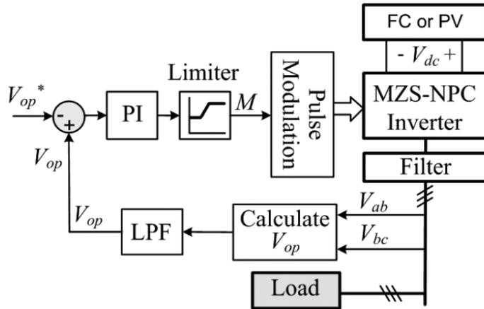
**Fig. 7.** Recommended closed loop control diagram of AC load voltage for MZS-NPC. MZS-NPC, modified Z-source neutral-point clamped.
