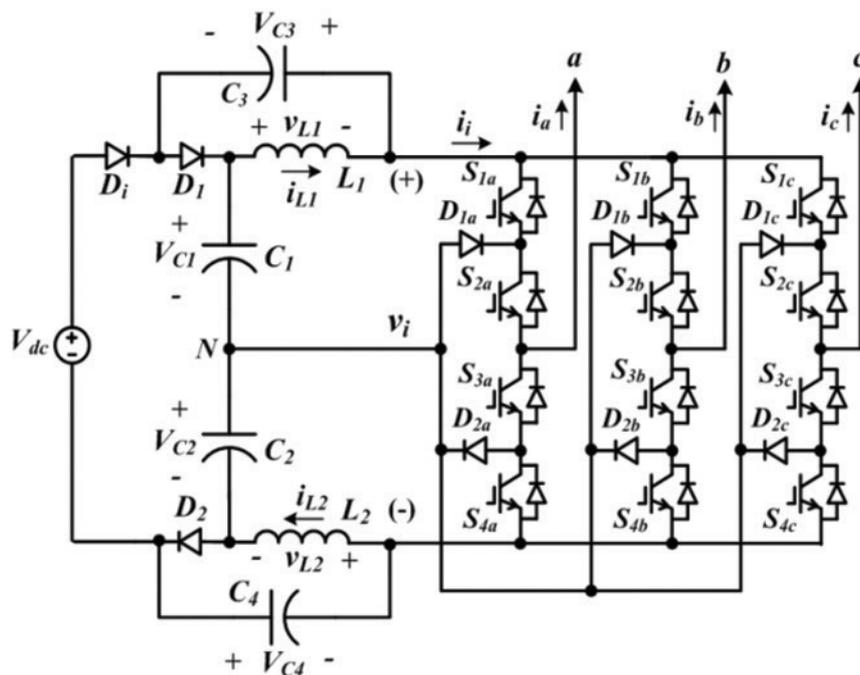
Fig. 1. Modified three-phase impedance source NPC inverter Strzelecki (2006). NPC, neutral point clipper.
