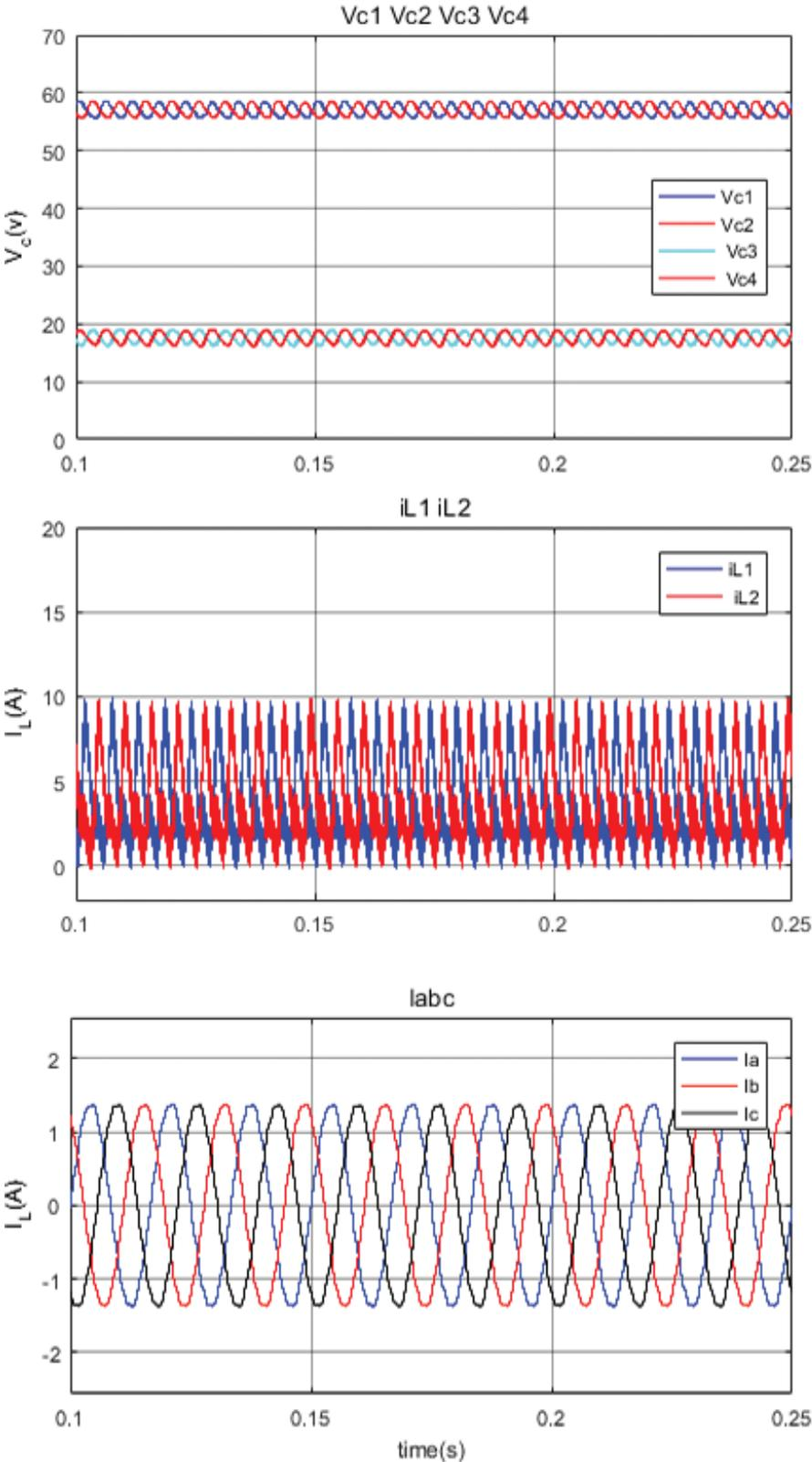
Fig. 12. The voltage waveform of capacitors and inductors and load current in  $M = 0.9$ .
