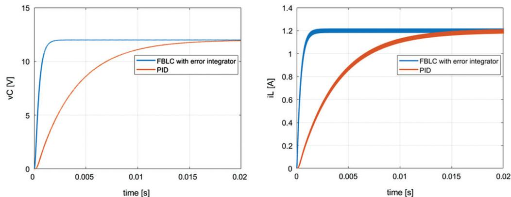
**Fig. 3.** Capacitor voltage and inductor current during start-up.
