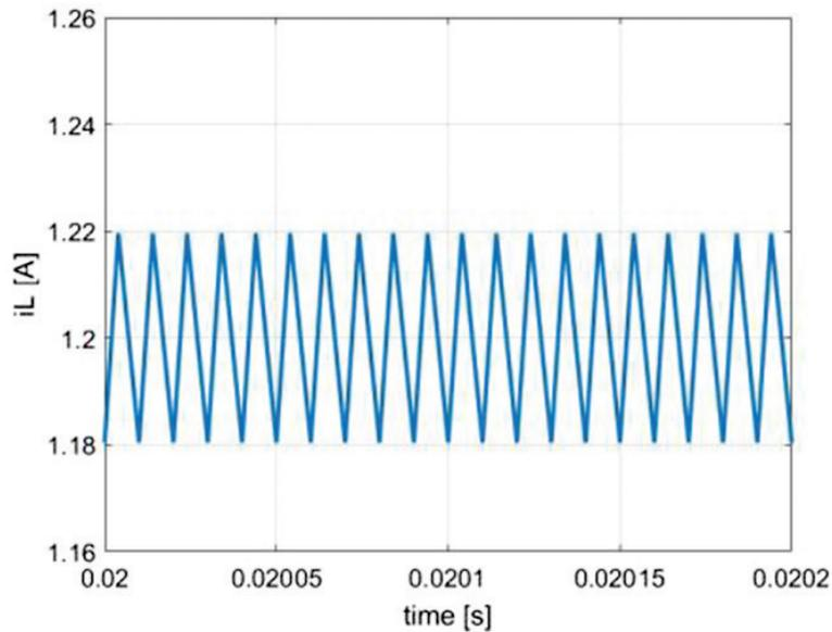
Fig. 4. Inductor current ripple in nominal condition (FBLC). FBLC, Feedback linearisation control.
