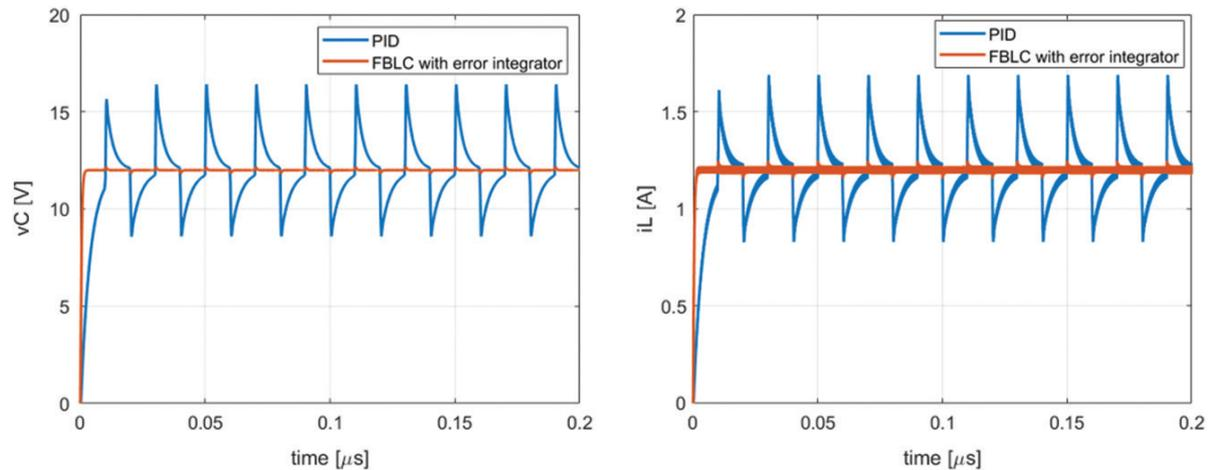
Fig. 6. Capacitor voltage and inductor current response to input voltage changes.
