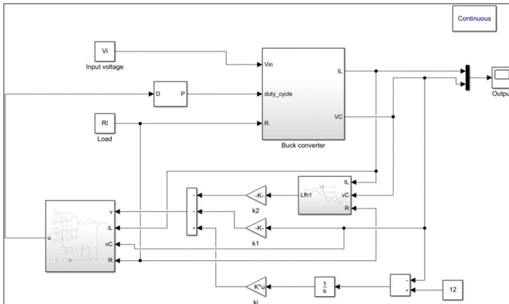
Fig. 2. Matlab Simulink model of the system with error integrator.
