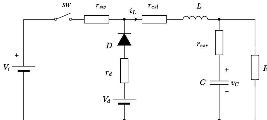
Fig. 1. Buck converter including parasitics.
