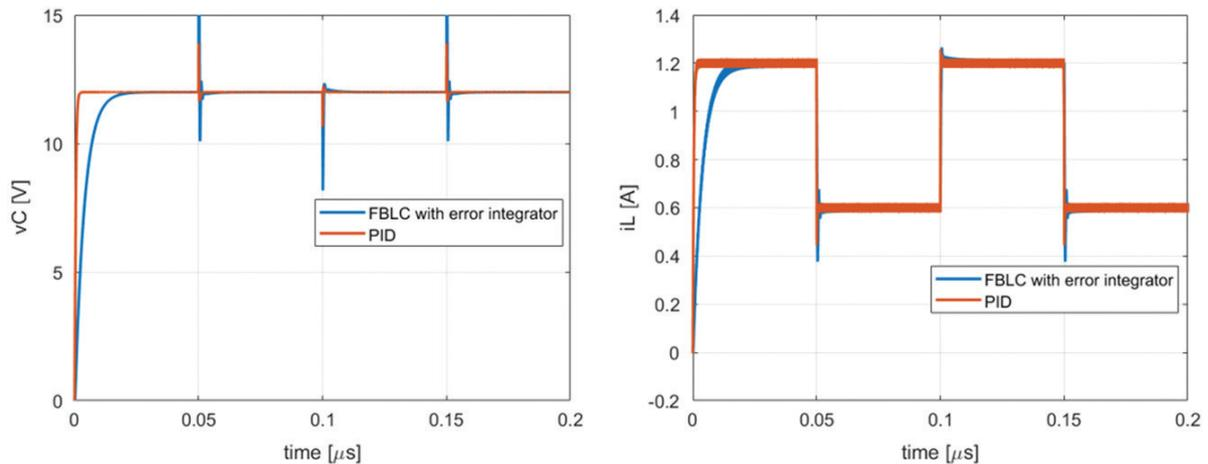
Fig. 5. Inductor current and capacitor voltage response to load changes.
