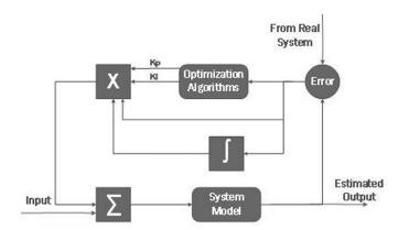
Fig. 5. Schematic diagram of the proposed observer's structure.
