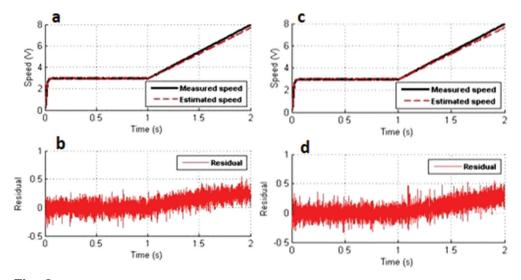
Fig. 9. Incipient fault case: (a) measured speed and estimated speed, (b) residual by the proposed observer, (c) real speed and estimated speed and (d) residual by Luenberger observer.
