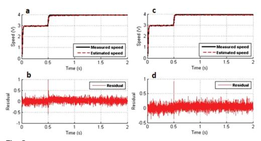
Fig. 8. Abrupt fault case: (a) measured speed and estimated speed, (b) residual by the proposed observer, (c) real speed and estimated speed and (d) residual by Luenberger observer.
