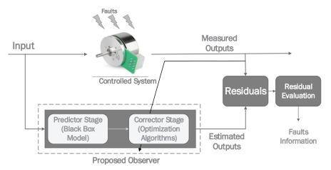
Fig. 1. Schematic diagram of the proposed observer-based FD approach.
