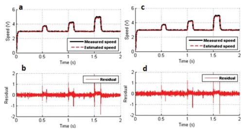
Fig. 10. Intermittent fault case: (a) measured speed and estimated speed, (b) residual by the proposed observer, (c) real speed and estimated speed and (d) residual by Luenberger observer.
