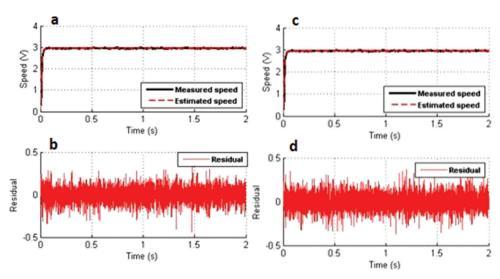
Fig. 7. Normal case: (a) measured speed and estimated speed, (b) residual by the proposed observer, (c) real speed and estimated speed and (d) residual by Luenberger observer.
