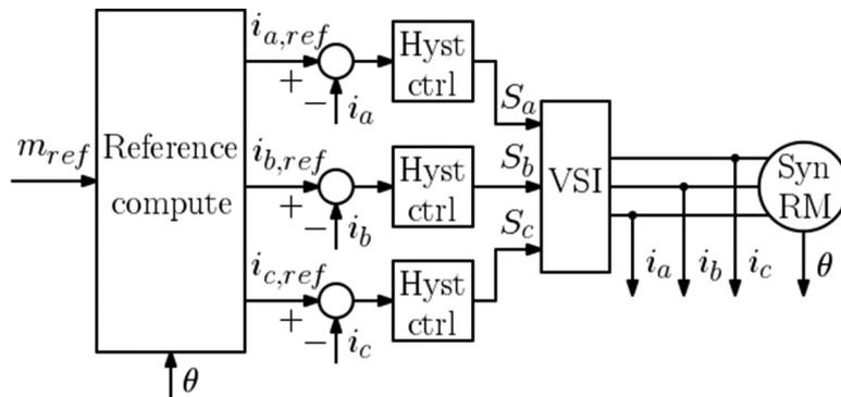
**Fig. 4.** Phase-current-based hysteresis current vector control (HCVC)
