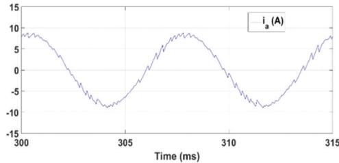
**Fig. 16.** A stator phase current in the steady state in the case of the HCVC with a  $50 \mu\text{s}$  torque-control sample time
