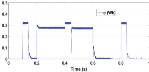
**Fig. 10.** The amplitude of the stator flux vector in the case of the HCVC with a  $20\ \mu\text{s}$  torque-control sample time
