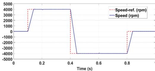
**Fig. 5.** The speed reference and the speed in the case of the DTC with a 20  $\mu$ s torque-control sample time
