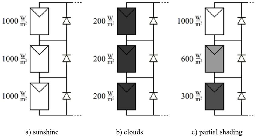
Fig. 4. Irradiance on PV panels in test scenarios
