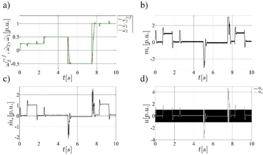
Fig. 4. Transients of angular velocities of the load (a), electromagnetic torque (b), shaft torque (c), and control signal (d); structure with the filter of constant bandwidth parameter  $m = 45$ , results of simulation
