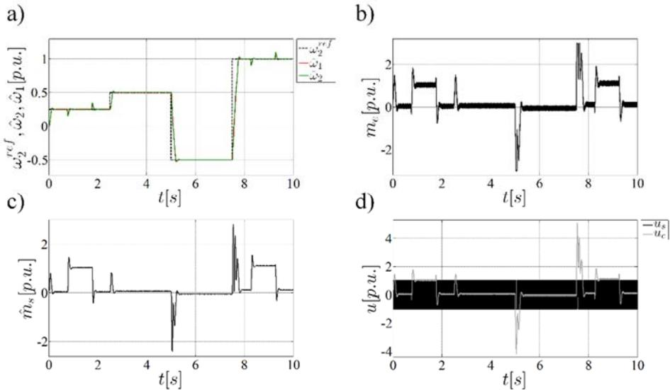
Fig. 5. Transients of angular velocities of the load (a), electromagnetic torque (b), shaft torque (c), and control signal (d); structure with the filter of constant bandwidth parameter  $m = 140$ , results of simulation
