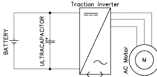
Fig. 1. Basic parallel topology of the HESS
