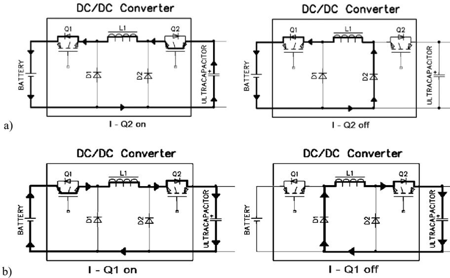
Fig. 8. Current flows in DC/DC converter:
