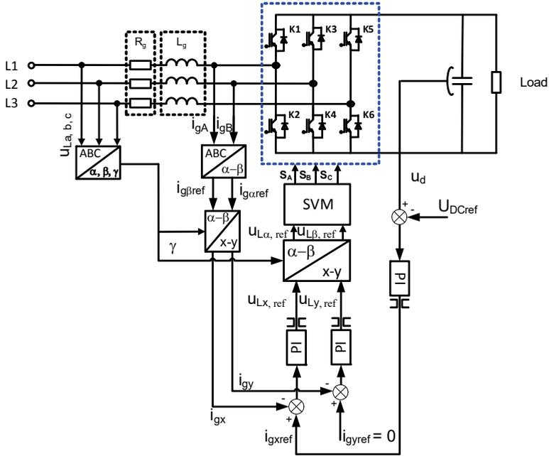
Fig. 12. Schematic diagram of Voltage Oriented Control (VOC)
