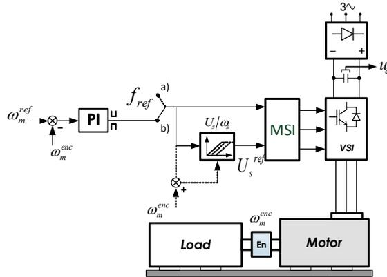
Fig. 5. Schematic diagram of a scalar structure of motor speed control:
