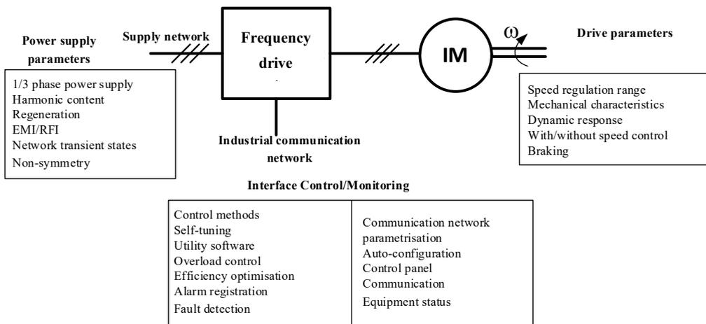
Fig. 14. Functions of a modern, regulated drive
