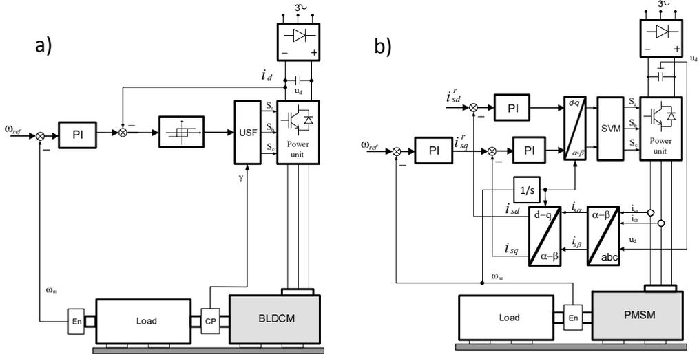
Fig. 11. Schematic diagram of inverter drive systems with synchronous motors:
