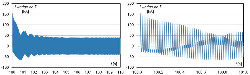
Fig. 8. Current waveform in the rotor wedge no. 7
