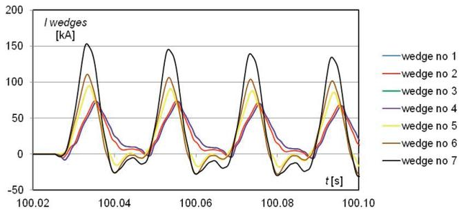
Fig. 9. Current waveforms in the rotor wedges
