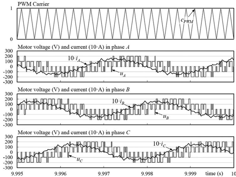
**Fig. 4.** Exemplary simulation outputs presenting PWM transients (at  $p\omega = 2100$  rad/s)
